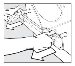
■ Remove the two struts together with the support plate.
